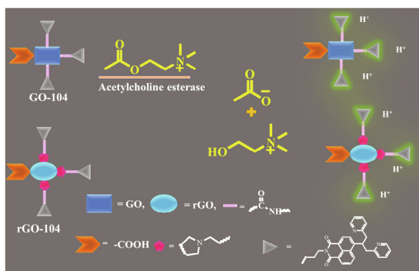
Fig. 89. Sensing of Ach by GO-104 and rGO-104.
